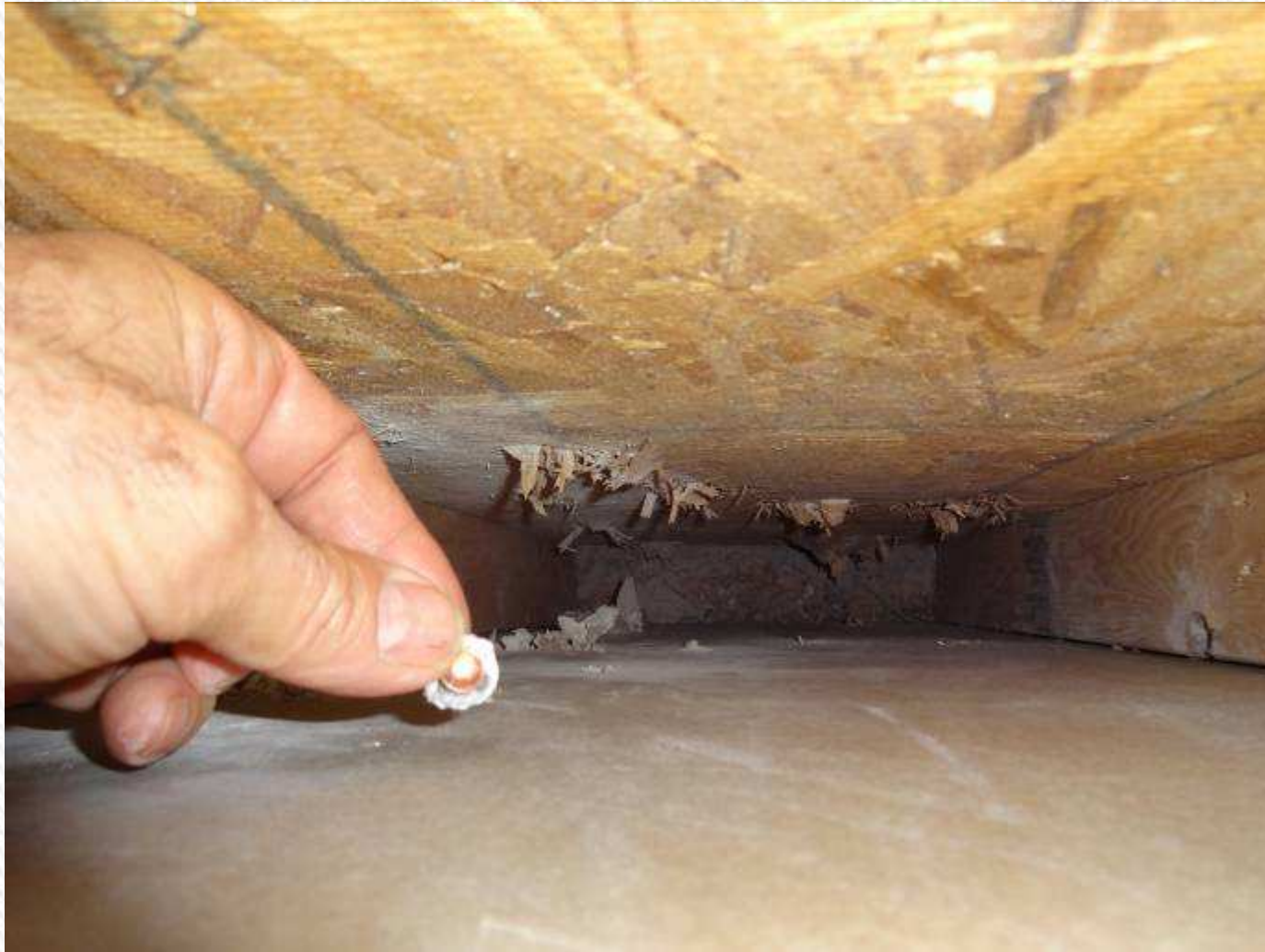
AK-47 bullet inside the wall after hitting BallistiCrete
