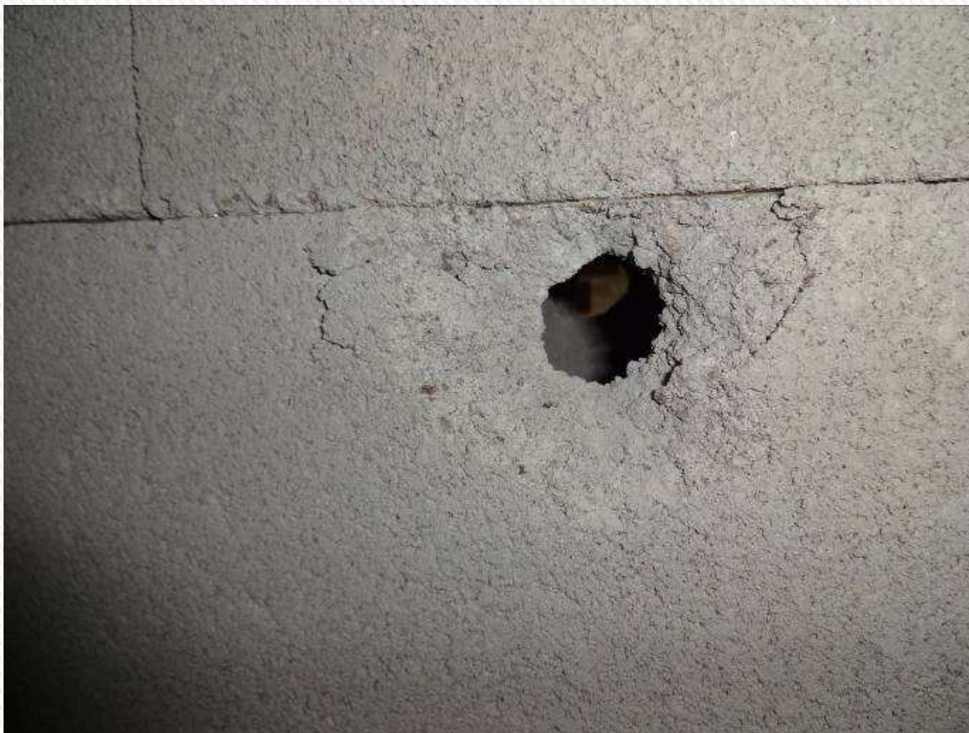
AK-47 exit hole on cement block, note the hole straight through.
