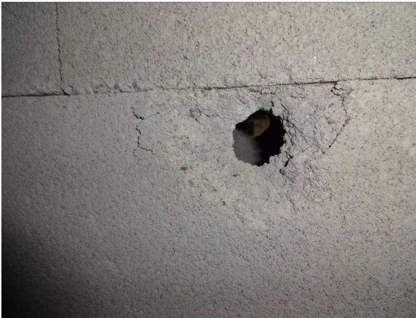
**AK-47 exit hole on cement block, note the hole straight through.**
