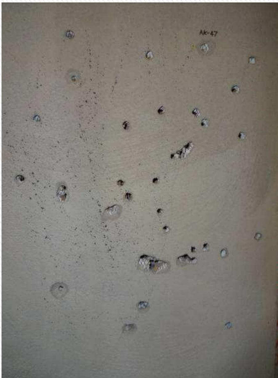
**Front side of a typical 3 coat stucco over OSB and 2x4 wood stud construction with gypsum board on the interior side.**
