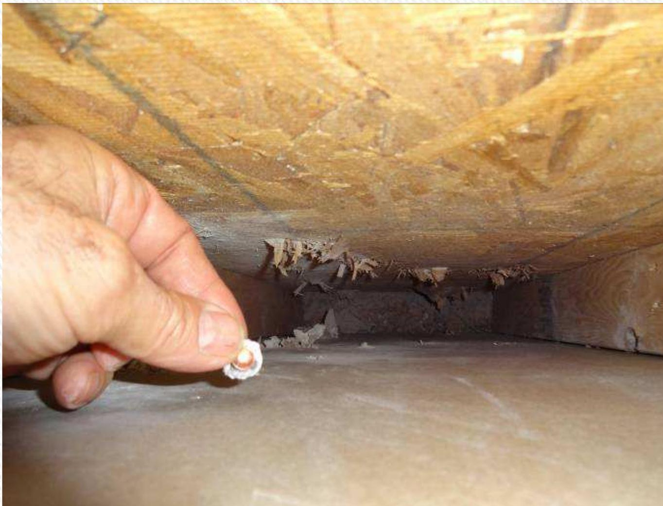
**AK-47 bullet inside the wall after hitting BallistiCrete**
