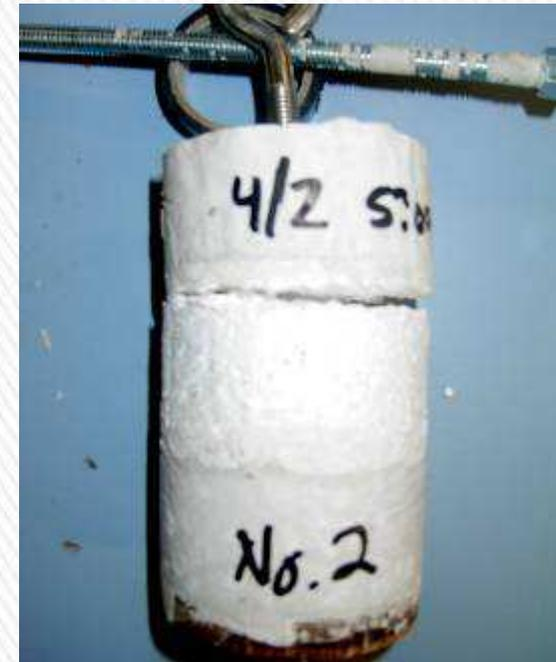
Bond strength to EPS foam always fails at the foam not the interface
